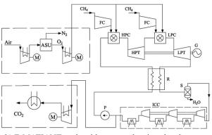
b) E-MATIANT cycle with two combustion chambers
