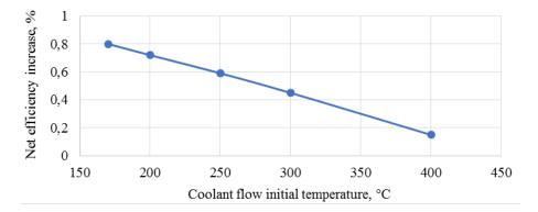
Figure 5 An influence of the coolant flow initial temperature on the net efficiency increase of the E-MATIANT cycle
