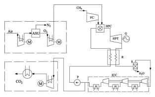
a) E-MATIANT cycle with one combustion chamber
