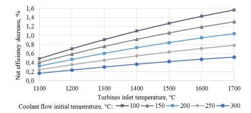
**Figure 4** An influence of the turbine inlet temperature on the E-MATIANT cycle net efficiency for the different coolant flow initial temperature
