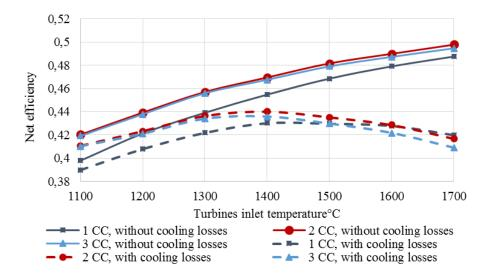
Figure 3 Turbine inlet parameters influence on the E-MATIANT cycle net efficiency with/without cooling losses
